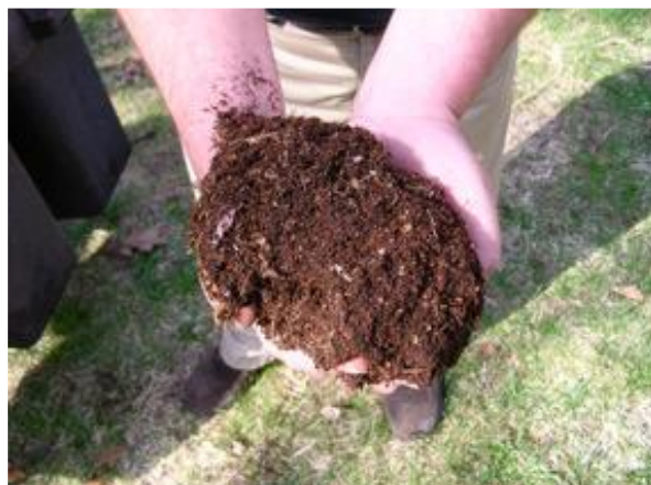
Figure 7. Compost, an example of an organic amendment used for green infrastructure projects. Image by Norman ack.
